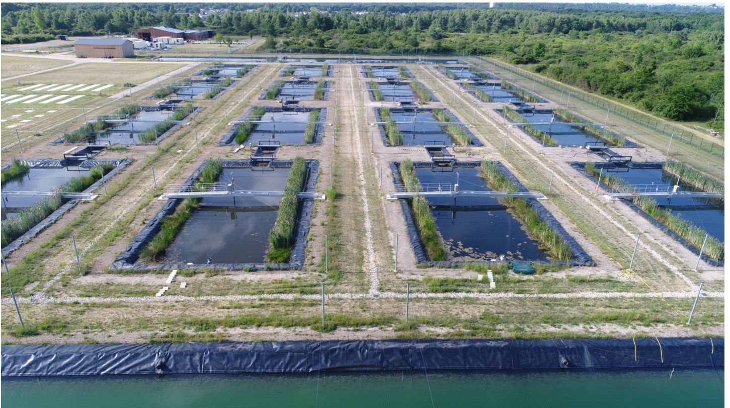
Figure 1: Macrocosms platform. 4 rows of 4 lakes oriented north-south. Storage lake on the south and drainage lake on the north
